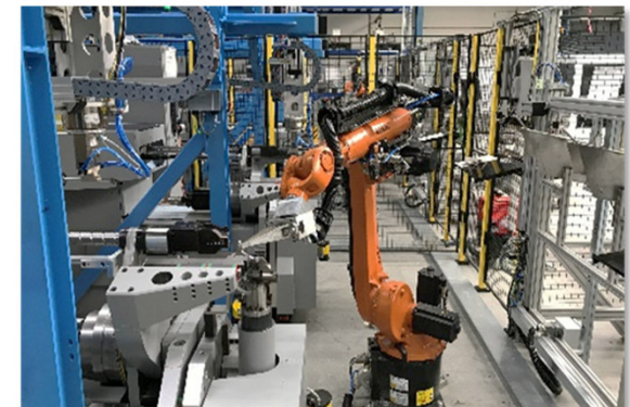
Inductive brazing process for example with studs and brackets at the end (as shown with bended tubes – or also brazing with straight tubes in front of bending process)
