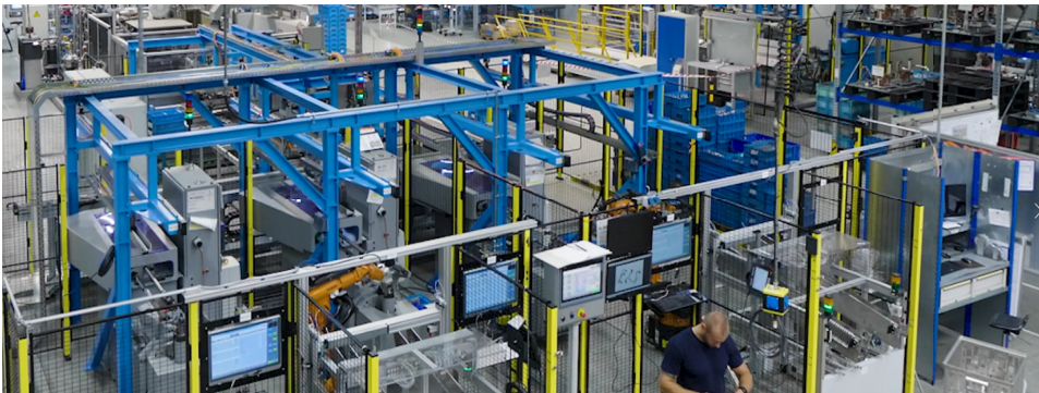
Fully Automatic Production line for: End forming | Roller finishing | 100% Camera check | Assembly nuts | Pre-cleaning | Annealing | Cool down and handling | Bending and handling
