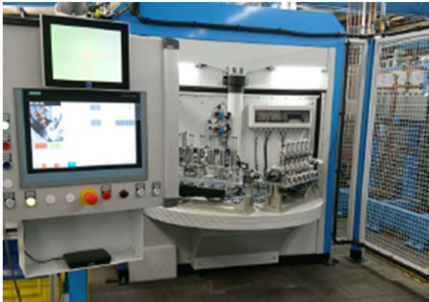
Laserspot- / Laserwelding cell with special clamping tools for exact welding results
